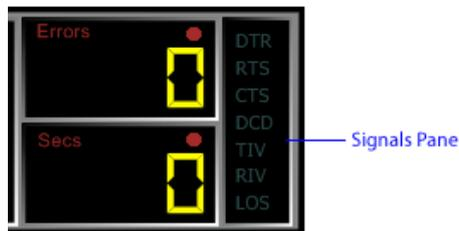
The FarSync BERT's current DTE signal states are displayed in the Signals Pane. Clicking the DTR and RTS indicators will toggle their output states.
