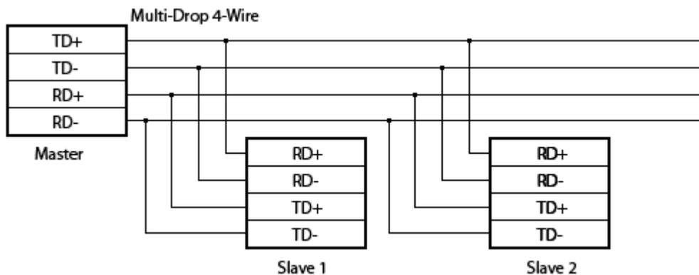
In the 4-Wire configuration, if a slave's RD+ and RD- wires have been incorrectly wired, the slave won't be able to detect messages addressed to it. If a slave's TD+ and TD- wires have been incorrectly wired, it won't be able to echo the data back successfully.
