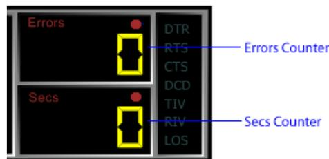
Pressing the **Errors** button (as shown in the diagram below) causes the **Errors** counter to switch between **BIT**, **BLOCK**, **SECONDS**, **PARITY**, **FRAME** and **ALL** error counter values.
