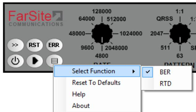
The **Reset To Defaults** menu option can be used to completely reset **all** the FarSync BERT's configuration parameters back to their factory default values.
