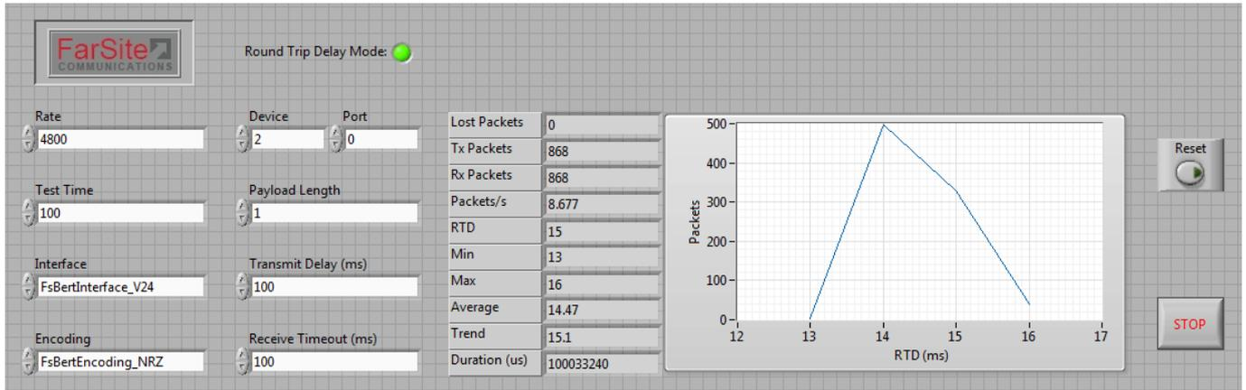
The Round Trip Delay VI sample demonstrates the features of the FarSync BERT's Round Trip Delay Mode.
