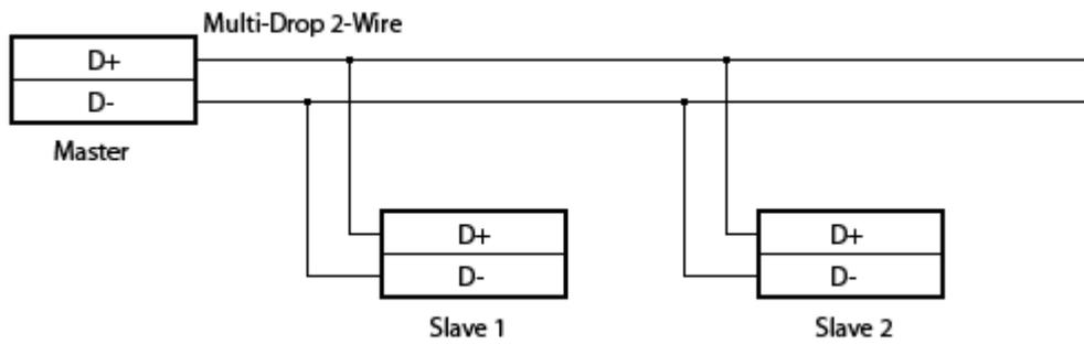
In the 2-Wire configuration, if a slave's D+ and D- wires have been incorrectly wired, the slave won't be able to detect and echo back packets which have been addressed to it and therefore won't be able to achieve sync.
