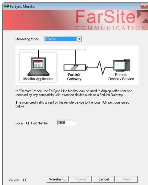
After configuring the TCP port, restart the line monitoring by pressing the "Record/Stop" button twice. You will then be able to view the monitored data from the FarLinX Connect Mini, in real-time. See Section 9.4 - Monitoring the HDLC lines using Wireshark, for details of how to monitor and analyse the data using the popular Wireshark network monitor application.
