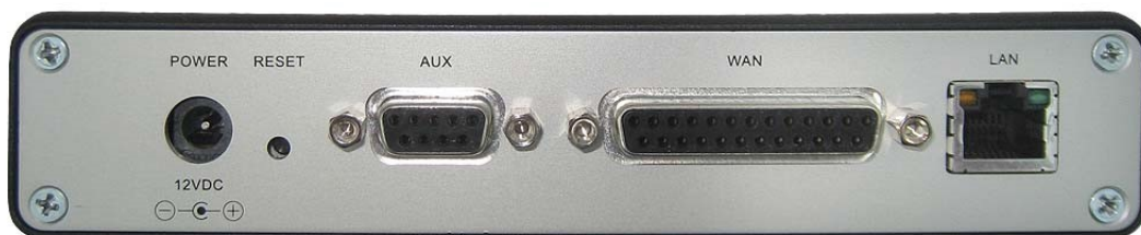
Rear panel view showing, 12V, 1.5A power input, system reset button, AUX port (not used), WAN port for the HDLC connection and a LAN connection
