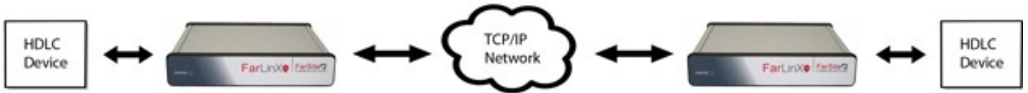
Diagram illustrates an HDLC connection being bridged over the TCP/IP network such as the Internet using a FarLinX Connect Mini at each end
