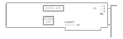
Jumper J4 is used to set the IRQ to 2, 3, 4, 5 or 7 by moving the jumper to the required position. The numbers above the jumper pins correspond to the IRQ number. Default setting is IRQ 5.
